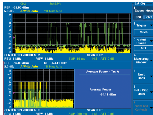
Example of burst and average power measurement with synchronous trigger
